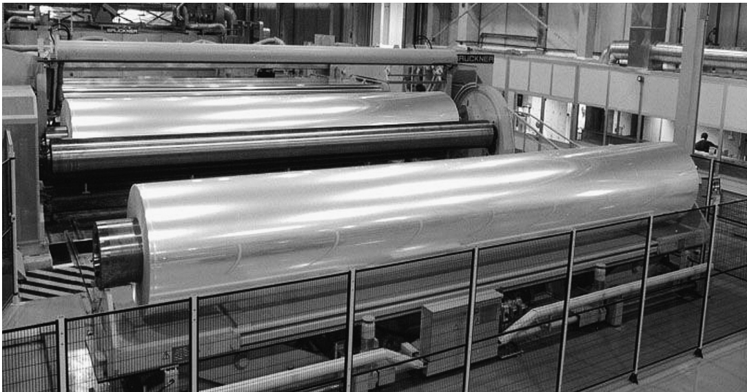
Figure 12.9 Finished 10-m BOPP mill.
